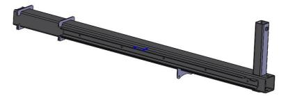
1. Begin by locating the ¼" x ½" set screws and screw them into the track support brackets from the rear until they are buried in the nut but not protruding out the front side of the nut.
